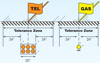
The facility at left is marked as being 20" wide. So, 24" on each side, plus the width of the facility, gives us a tolerance zone of 68".
